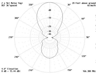
The front-to-back ratio is now close to 9dB, the gain has dropped about 2.8dB which would cause a reduction of detection distance of almost 28% in the direction the yagi is pointed.
