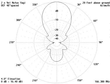
The front-to-back ratio is now close to 13dB, the gain has dropped about 1.8dB which would cause a reduction of detection distance of almost 19% in the direction the yagi is pointed.
