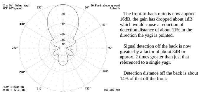
Recommendations: If only two yagis are to be used at a site, and they are to be oriented 180° apart, a minimum recommended spacing should be 60" (1.52m). There will be approx. 10% reduction of forward gain of both yagis, plus detection off the back of each yagi will be degraded by about 14%.
