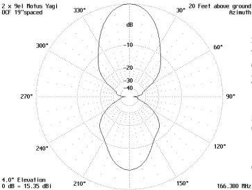
Besides the obvious loss of front-to-back ratio, the forward gain has dropped about 3dB which would cause a reduction of detection distance of almost 30% in the direction the yagi is pointed.
